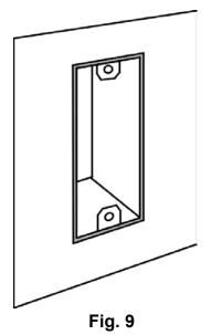
NOTE: Always move the cutting bit in a **counter clockwise** direction around the outlet box. The natural tendency of the cutting bit to move to the left will make it easier to cut close to the box.
